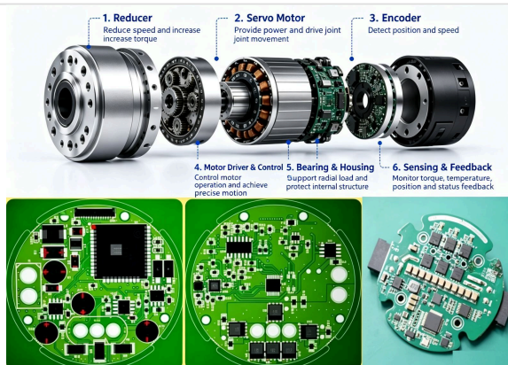
Integrated Joint Module · Exploded View & Controller PCB
